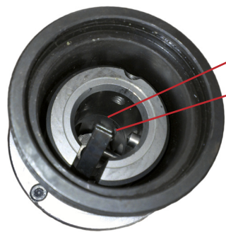
Wear/damage in ID of shank
